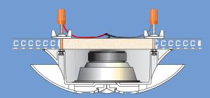
Two standard wire nuts connect the speaker wires to the studs – and that's all it takes!
