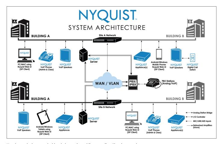
Nyquist can be integrated with existing analog cabling as well as IP-only networks
